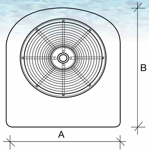
Minimum Clearance required to wall or obstruction 60cm
