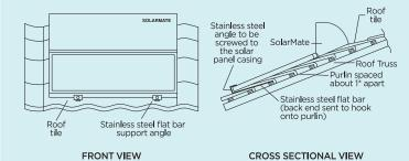
Details of dimension, sizes and number of stainless steel flat bar support angle straps required for SolarMate are as shown for the 2 models:
