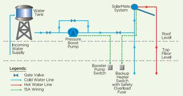
\*Take note that SolarMate will cover wiring, cold water inlet and hot water outlet of SolarMate up to 3 meter each only.
