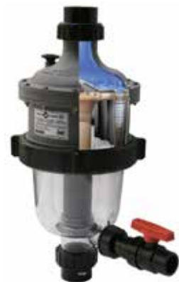
The MultiCyclone M16 is a pre-filtration device that works on the basis of centrifugal water filtration. There are no moving parts to wear and tear and no filter media to clean or replace.
