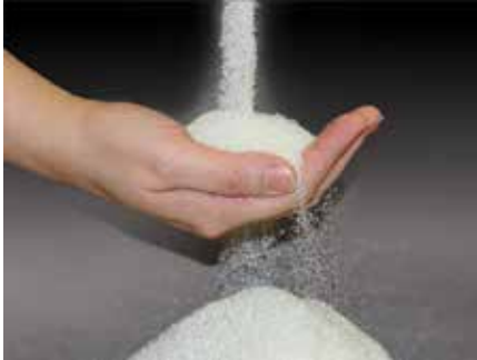
Waterco's Glass Pearls are manufactured from 100% pure glass and offer much finer filtration than conventional filter media.
