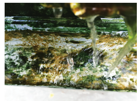
Algae build-up in one of the hydroponic drains that caused problems for the entire system.
