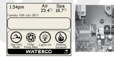
The Aquamaster system comes complete with one touch screen control. An additional screen available separately may be connected providing additional operational convenience to the owner. There is a small jumper link on the circuit board which must be removed.
