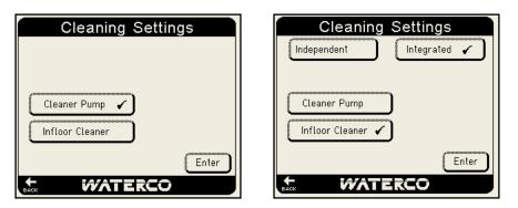
If the installed system is fitted with a Cleaner Pump select the "Cleaner Pump" icon and press "Enter".
