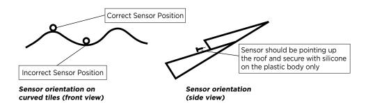
The sensor should be orientated such that it lies on the crest of the roof tiles and not in the troughs. This eliminates water being trapped in the silicon glue that holds the sensor in place, and giving erroneous readings. The roof sensor should also be positioned so that it points up the roof tiles (as shown above).
