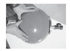
b. Wrap 3-4 turns of Teflon tape onto the male threaded end of the controller. Take the Pressure Pack and Tee Fitting and screw onto the pump controller.
